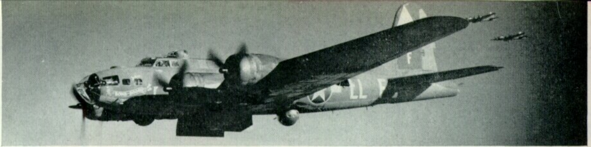
A late model B-17F "Bomb Boogie" of the 401st B.S., 91st B.G. with modified cheek gun position which allows .50 to fire directly forward. (Photo: U.S.A.F.)
