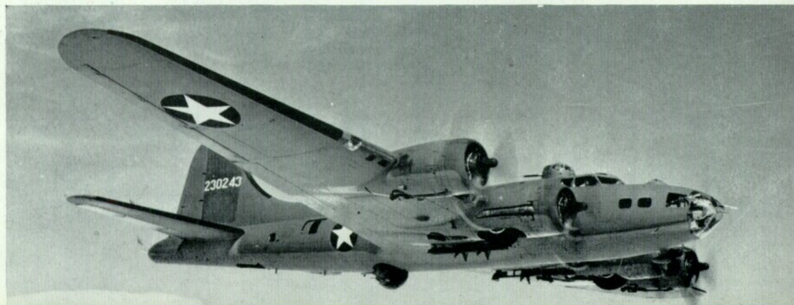
B-17F with external bomb racks in place on a test flight over Mt. Rainier, near Seattle, Washington.
