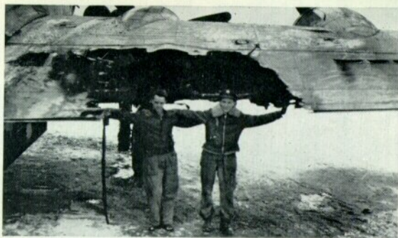
Battle damage 1: this Fortress returned to base safely after a burning wing tank had destroyed 30% of the wing root. (Photo: W. J. Connell collection)
