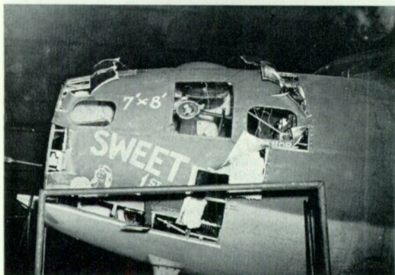
This unusual sequence graphically demonstrates the "repairability" of the Fortress. Top left shows "Eight Ball", a B-17E-25-DL (DO) of the 91st B.G., serial 42-3138, with nose damage from a runaway propeller. The area to be replaced is marked off with masking tape. Top right shows the section removed, with the replacement nose from "Sweet Pea 1st" ready. Bottom left shows the section in place. Bottom right shows job almost complete. (Photos: W. J. Connell collection)
