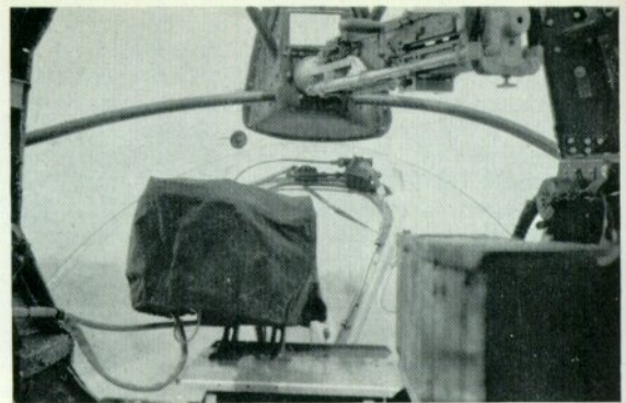
Navigator's eye-view of the single .50 cal. gun in the nose of a B-17F. In this case the installation appears to be a factory-supplied kit rather than a field modification. Note shrouded Norden bombsight. (Photo: W. J. Connell collection)
